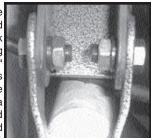
1/2" x 20 x 3-1/4" bolts, lock washers and nuts. Tighten all bolts.
