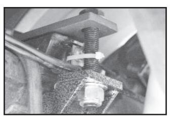
8) After installing the springs with the axle on to of the springs with the flit brackets u-bolt spring plate and top bracket is very straightforward except the break line brackets. Reusing the piece of the bracket that was cut reverse the bracket so the rubber break line mount is reversed. This is important so the bracket is against the bolt NOT the break line. A nylon tie does a good job securing the assembly in place.
