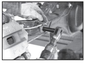
5) Relocating the break line bracket is very important. It must be done with care so the breakline is secure.
