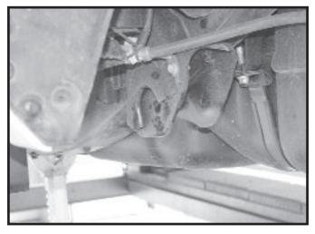
4) Completely remove the rear spring. Support the rear end with a floor jack. This will help maneuver the rear end . You can remove the stock shackles and replace with the new longer ones.
