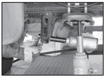
3) Completely remove the shocks. Again make sure the truck is supported properly you will have to lift both sides to perform the installation.
