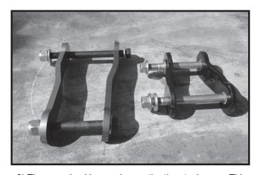
2) The rear shackles are longer the the stock ones. This will lift the truck, we used the longest hole distance on our installation.
