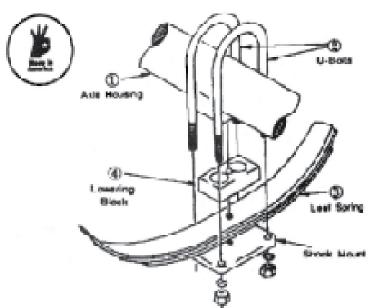
Doing one side at a time, remove the u-bolts. Using a hydraulic jack raise the axle away from the leaf spring and lower the axle down so the weight is on the block. Install and tighten the u-bolts evenly to 80ft lbs. Repeat the procedure on the other side of the truck. If there is excess u-bolts cut accordantly. It recommended to make a habit of checking tightness every few months
